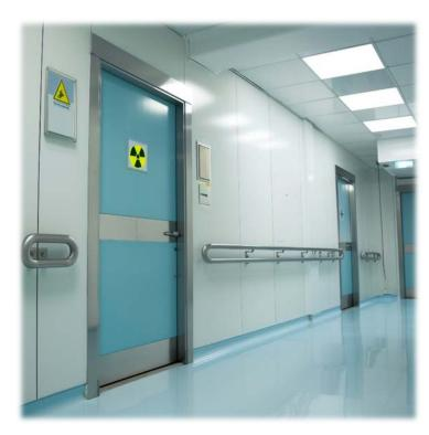
Our radiation doors are lead-lined and available with different lead thickness options to provide varying levels of radiation shielding. Thicker lead layers offer higher levels of protection, suitable for areas with higher radiation levels or specific regulatory requirements.
