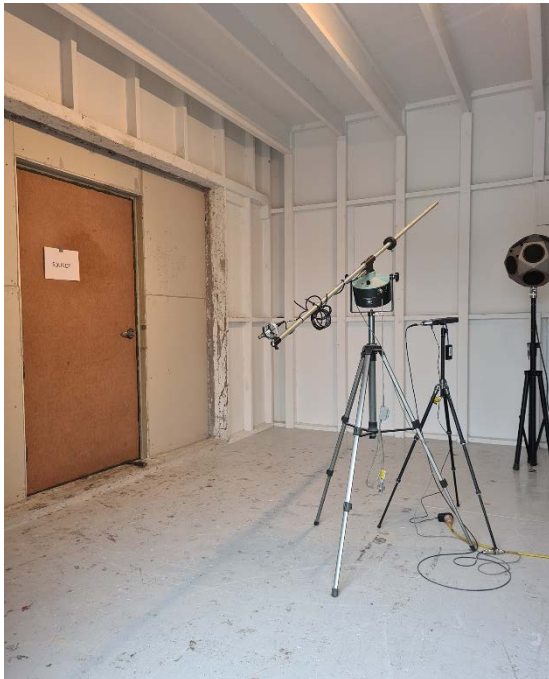
Image: SoundPro Door set undergoing acoustic testing
